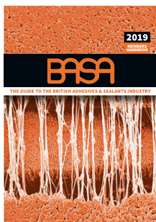
Cover image: sintered PTFE on an anodic oxide, tested to destruction. Copy right: Prof Gary Critchlow, Materials Department, Loughborough University.
